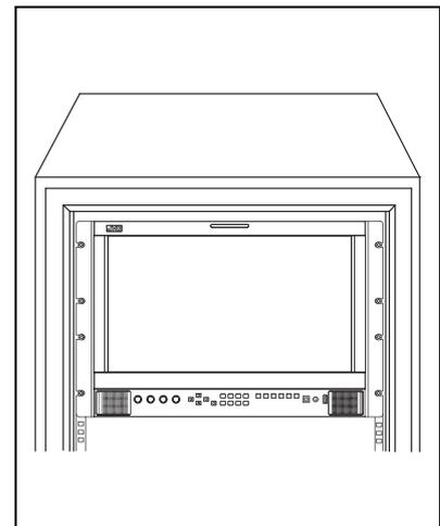
Step1: Fix the supplied rack ears onto left and right side of the DT-G17E monitor, by supplied 4 screws.
