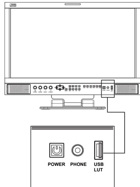
Insert the USB stick onto monitor USB port on the FRONT panel
